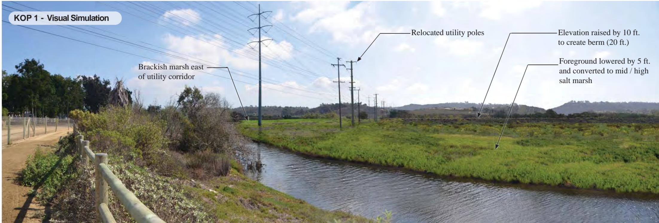
Note: It may be possible to relocate 2 electrical lines (12dV; 69Kv) onto other existing structures in the current corridor instead of constructing relocated poles. This represents worst -case, relocateddd pole configuration.
