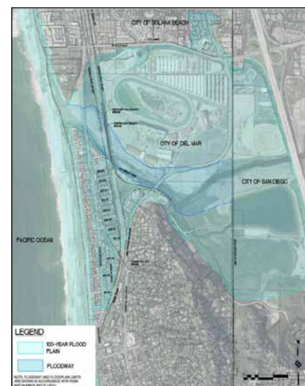
The rail bridge and track approaches are located in the FEMA 100-year flood plain. Source: FEMA
