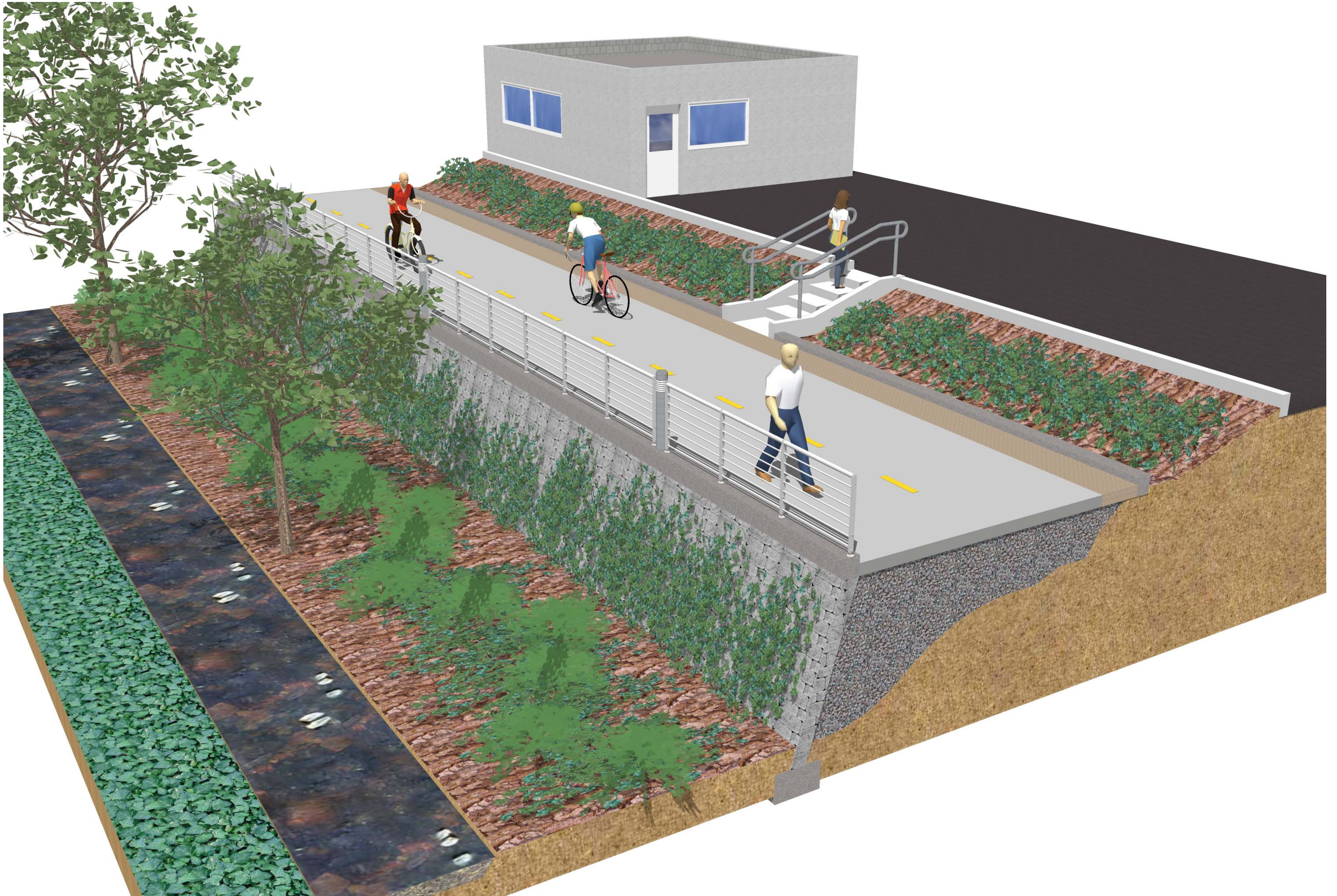
Oblique view of separated multi-use path
