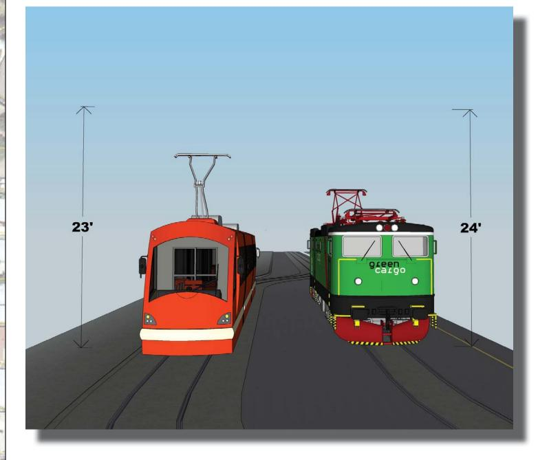
Minimum clearance required LOSSAN Railroad (LOSSAN): Aproximately 24' MTS Light Rail Transit (LRT): Approximately 23'
