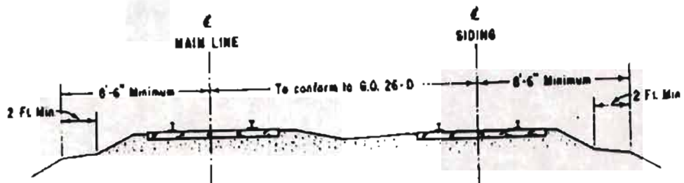
STANDARD No. 2 WALKWAYS ALONG MAIN LINE TRACKS
