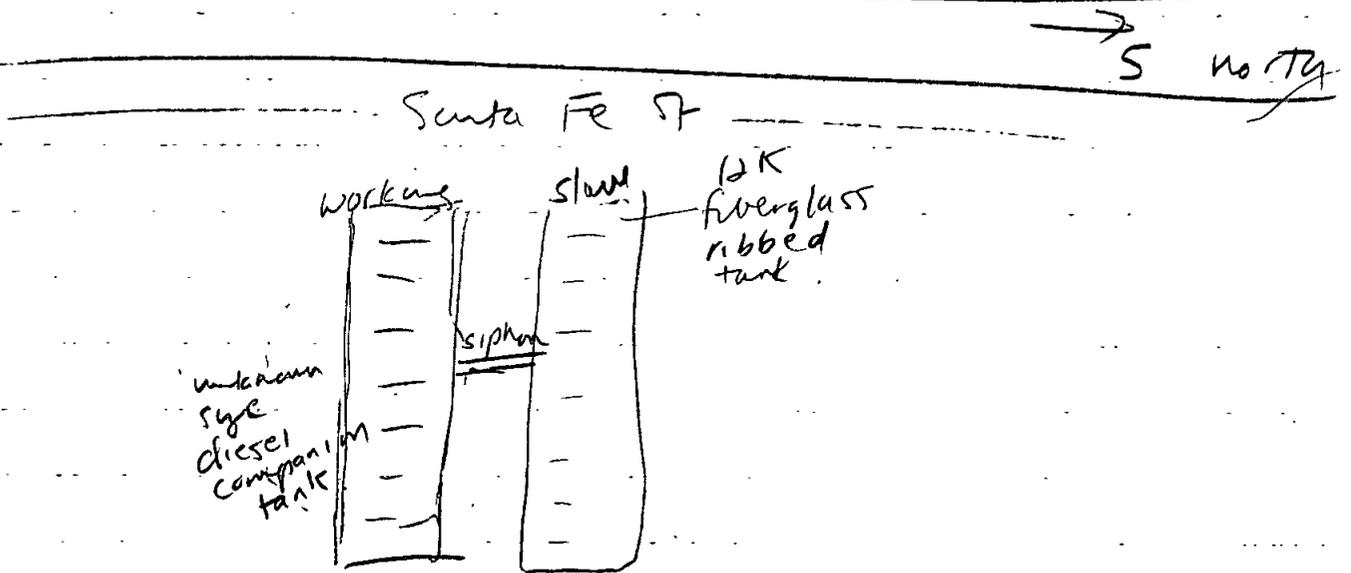
1115. Line snapped - line leading from dispenser to slave tank. Approx 10 g diesel poured onto ground. I asked Chris about the possible damage to the work tank. He did not think there was any damage.
