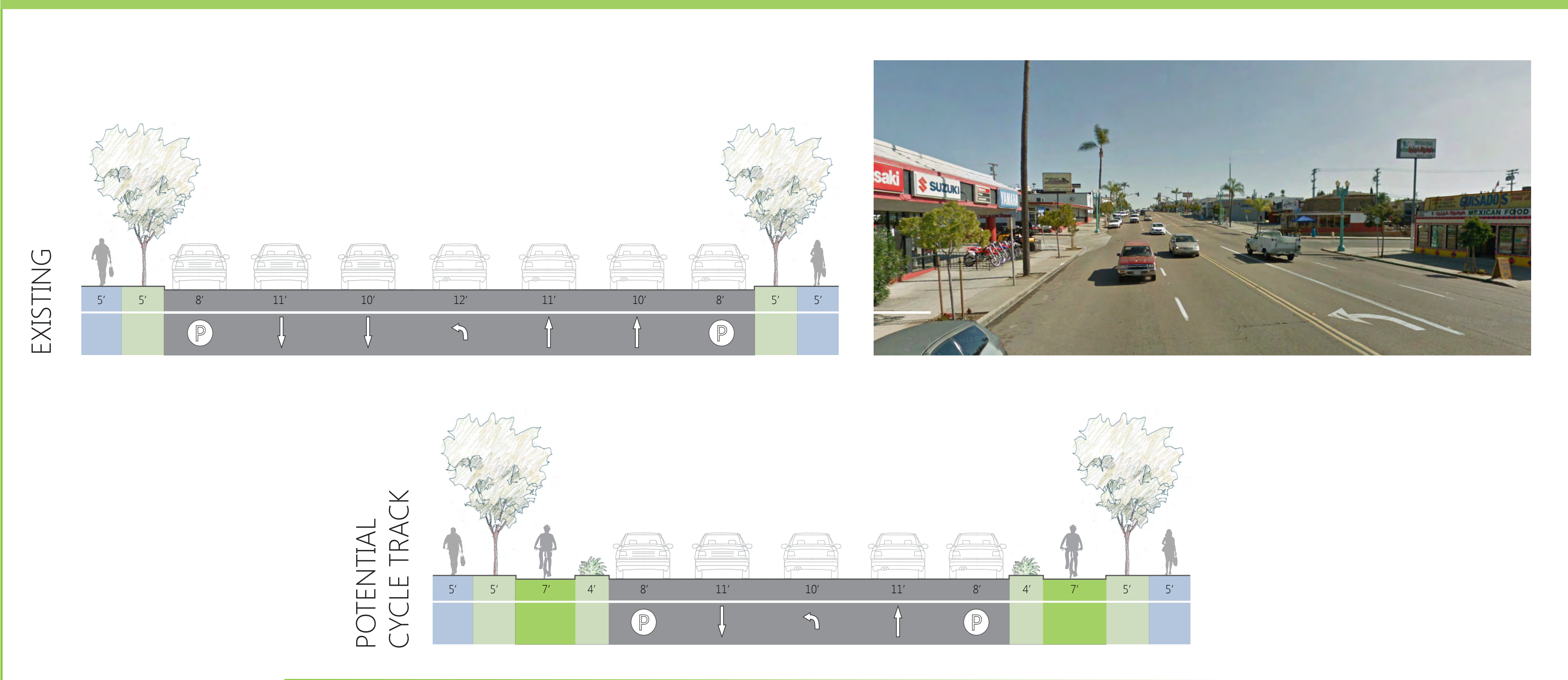
TYPICAL CROSS SECTION: EL CAJON BLVD BETWEEN FAIRMOUNT AVE & COLLWOOD BLVD
