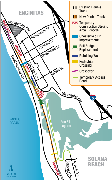
The project will add 1.5 miles of second main track and replace an aging timber rail bridge on the LOSSAN coastal rail corridor between the cities of Encinitas and Solana Beach.
