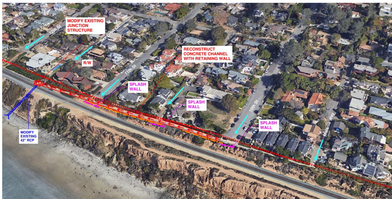
Figure 25 – Drainage Area 5 Improvements
