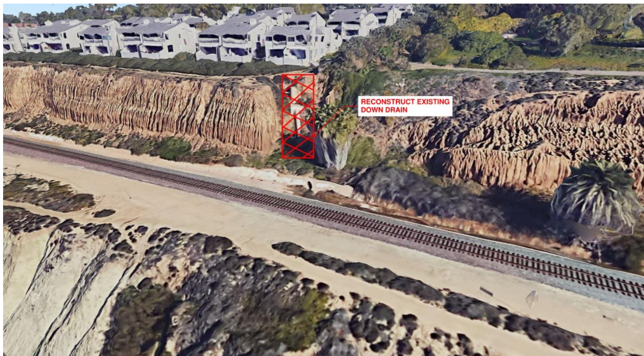
Figure 40 – Drainage Area 13 Improvements
