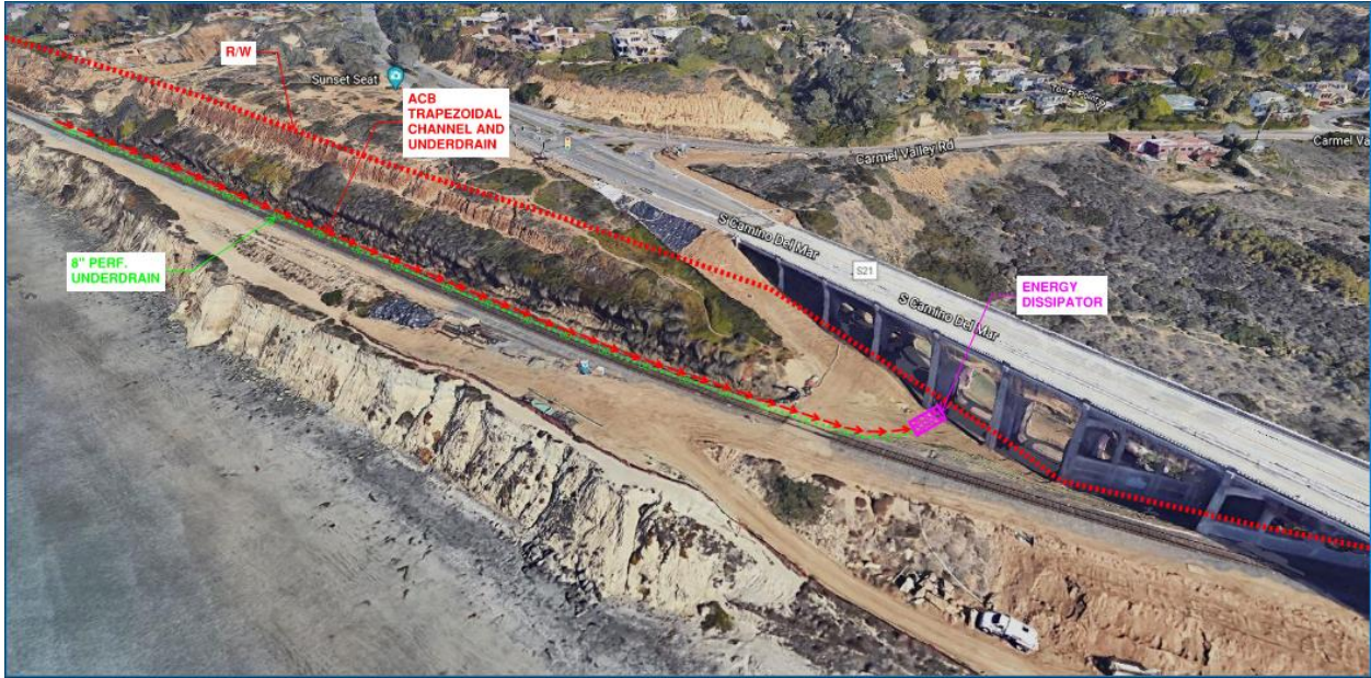
Figure 41 – Drainage Area 14 Improvements
