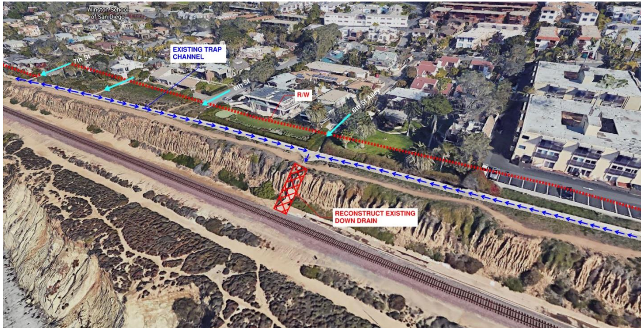
Figure 38 – Drainage Area 11 Improvements
