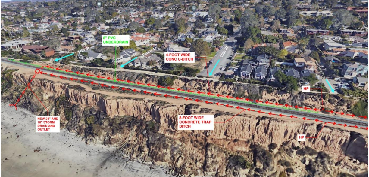
Figure 31 – Drainage Area 6 Improvements
