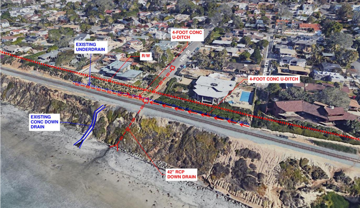
Figure 22 – Drainage Area 4 Improvements
