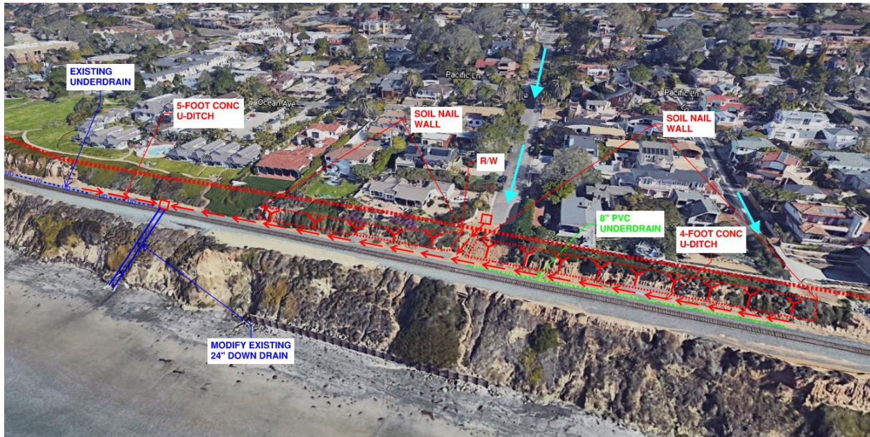
Figure 20 – Drainage Area 3 Improvements
