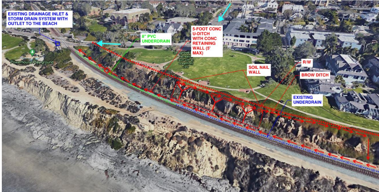
Figure 17 – Drainage Area 2 Improvements
