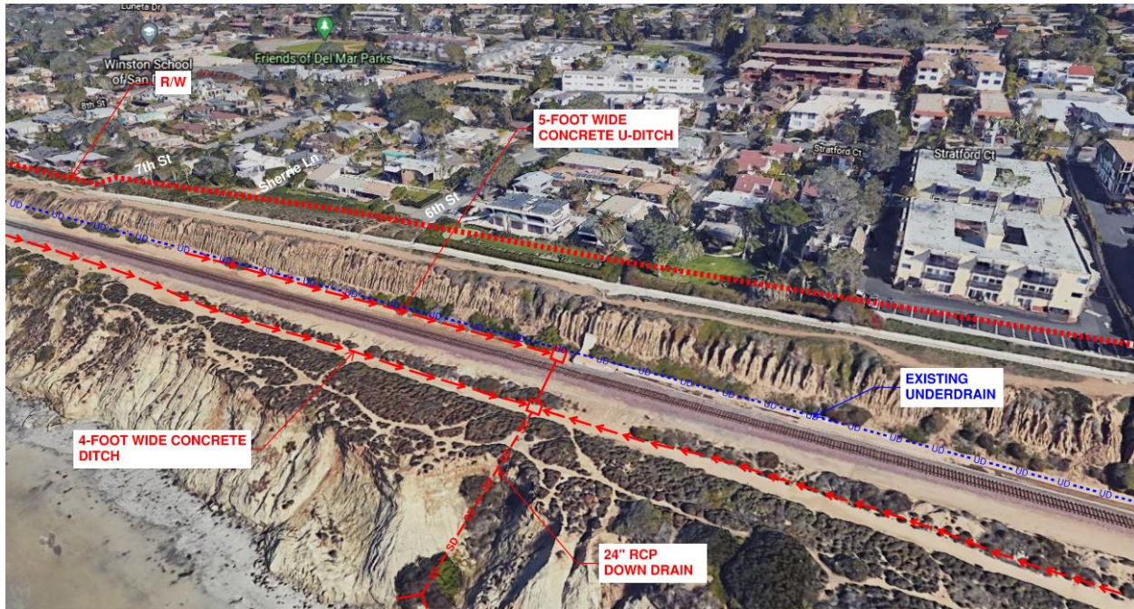
Figure 36 – Drainage Area 9 Improvements
