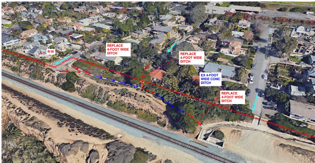
Figure 34 – Drainage Area 7 Improvements
