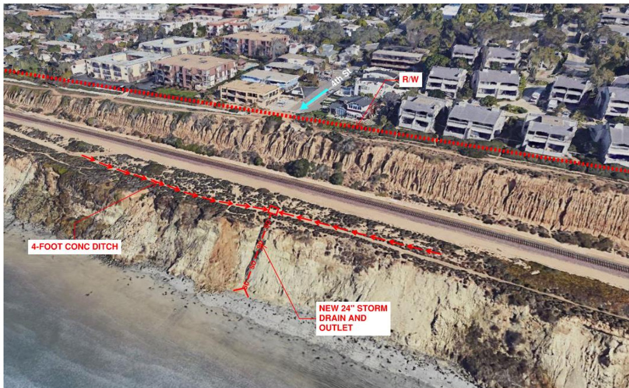
Figure 39 – Drainage Area 12 Improvements
