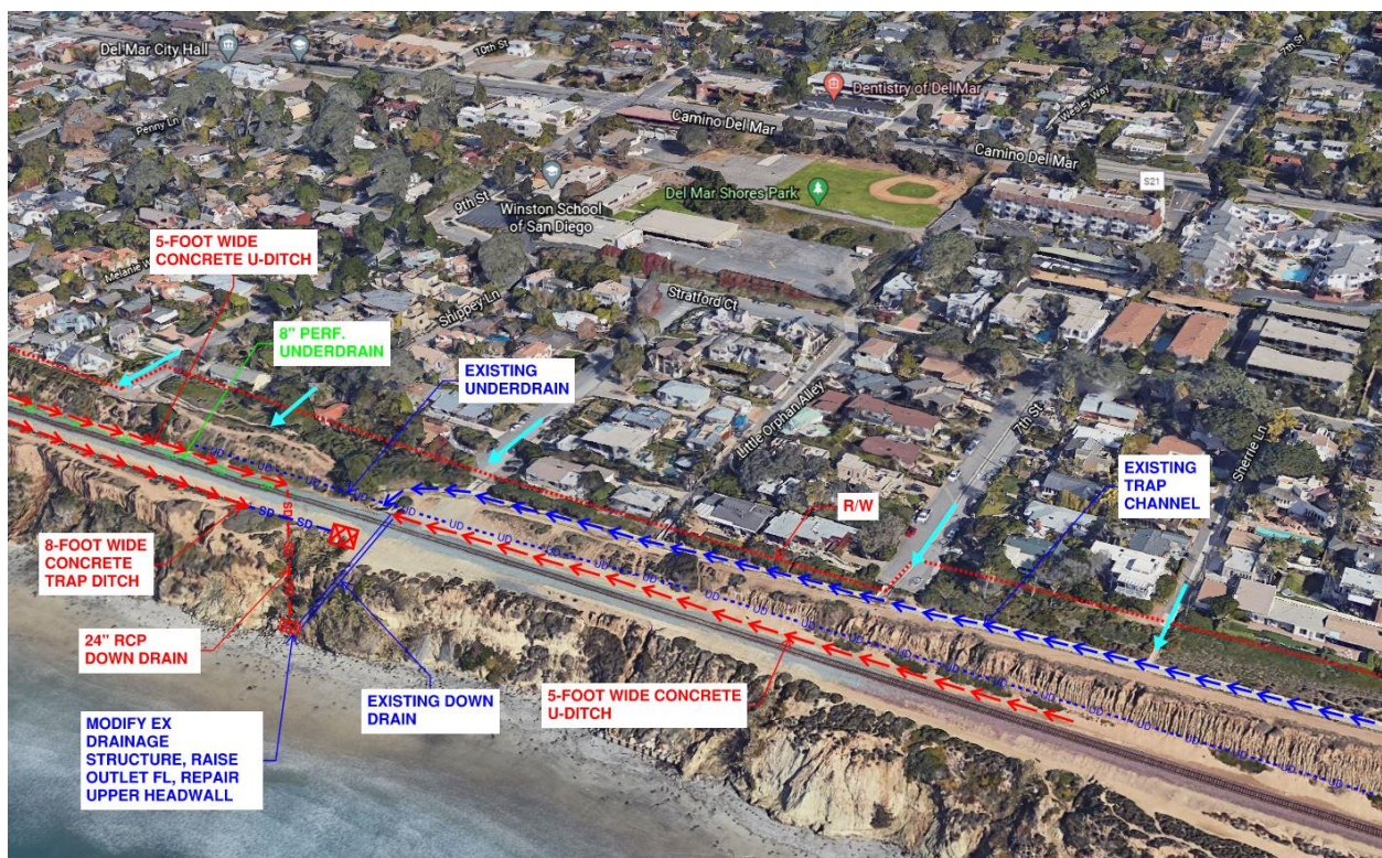
Figure 35 – Drainage Area 8 Improvements
