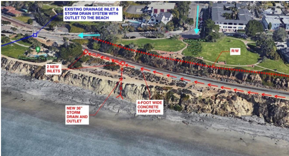
Figure 16 – Drainage Area 1 Improvements
