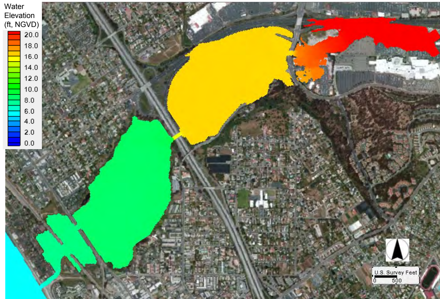
Figure 5.17 Maximum Water Elevations under Hybrid A during a 100-Year Storm in Year 2050
