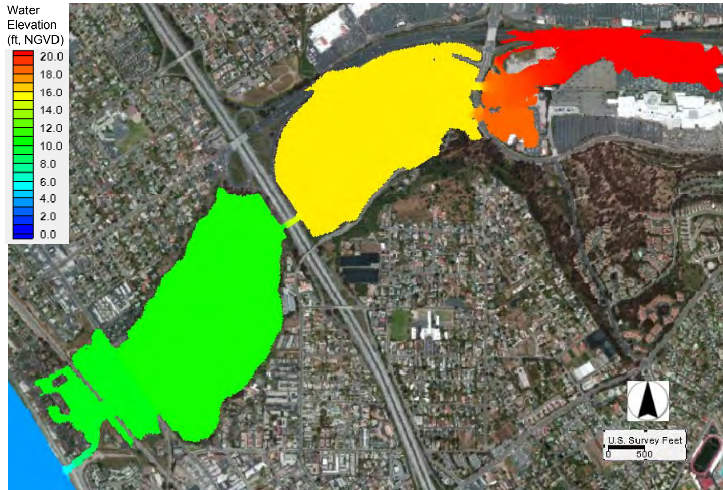
Figure 5.8 Maximum Water Elevations under Freshwater Alternative during a 100-Year Storm in Year 2015
