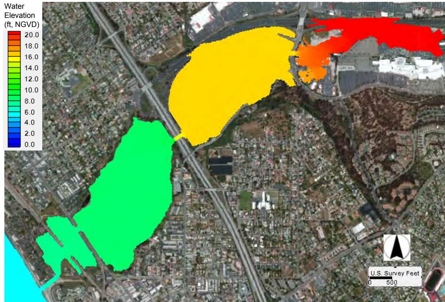
Figure 5.21 Maximum Water Elevations under Hybrid B during a 100-Year Storm in Year 2050
