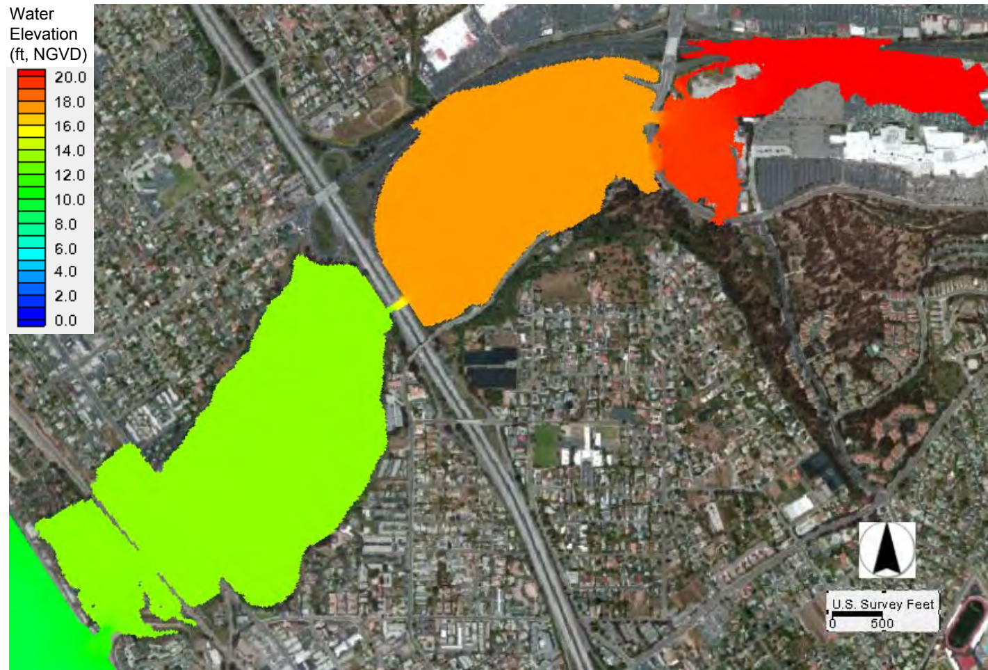
Figure 5.5 Maximum Water Elevations under No-Project Conditions during a 100-Year Storm in Year 2050
