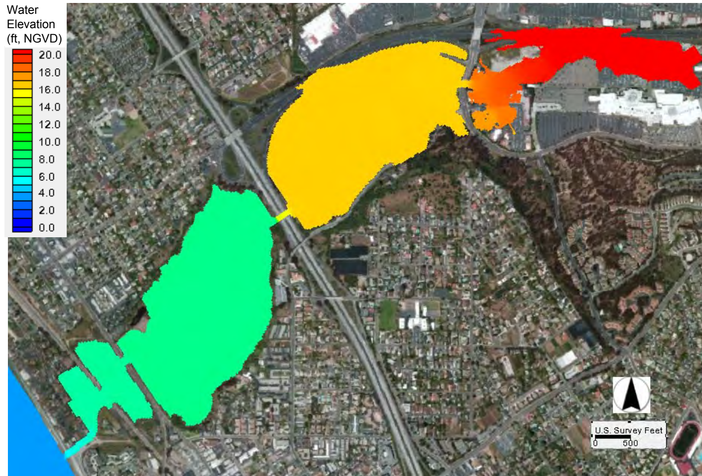
Figure 5.16 Maximum Water Elevations under Hybrid A during a 100-Year Storm in Year 2015
