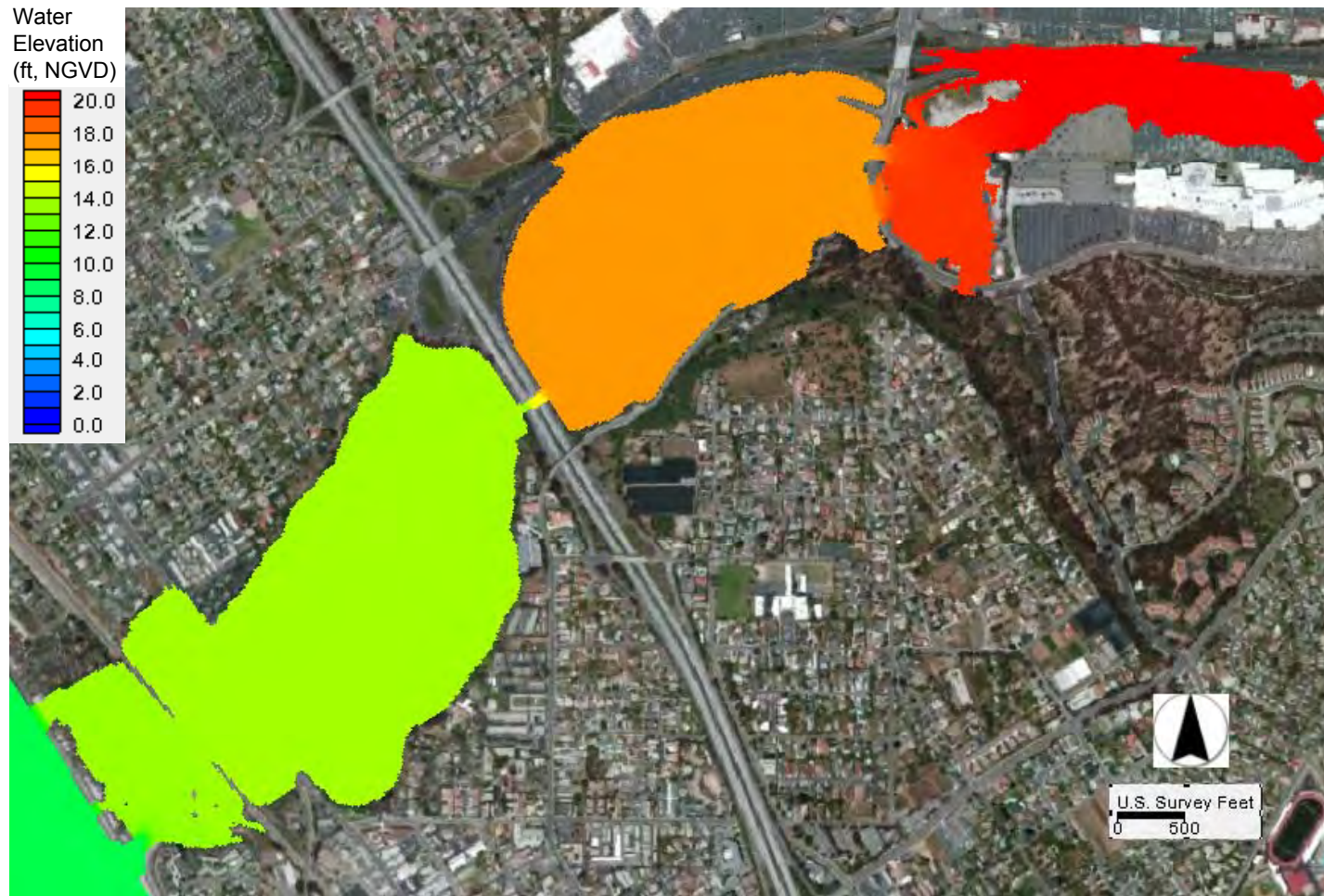
Figure 5.6 Maximum Water Elevations under No-Project Conditions during a 100-Year Storm in Year 2100
