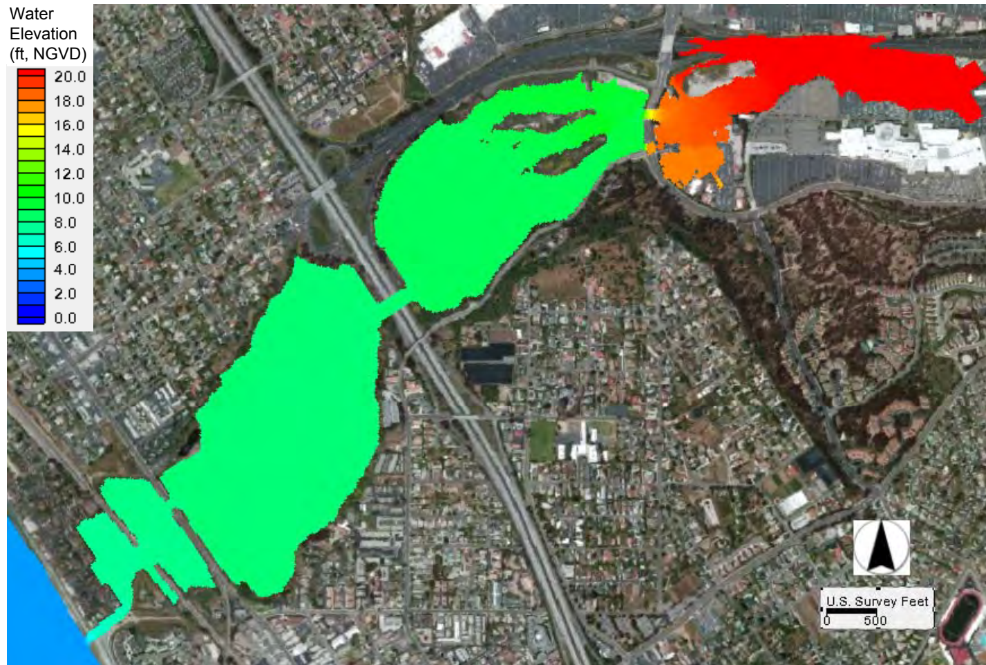
Figure 5.12 Maximum Water Elevations under Saltwater Alternative during a 100-Year Storm in Year 2015
