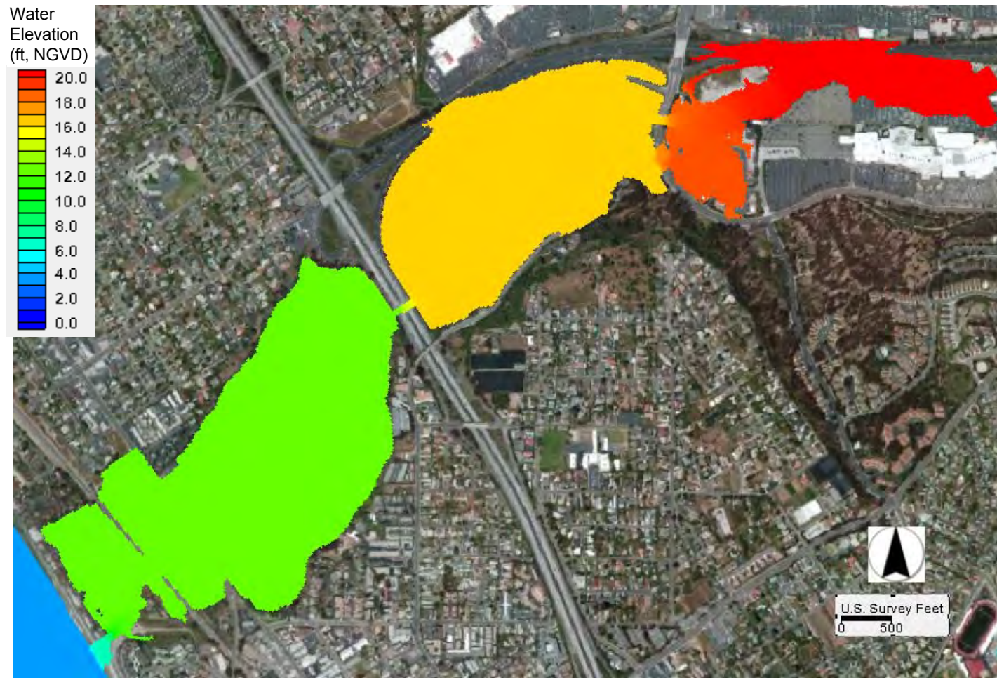
Figure 5.3 Maximum Water Elevations under Existing Conditions during a 100-Year Storm in Year 2015
