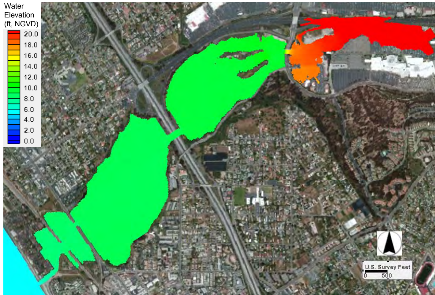
Figure 5.13 Maximum Water Elevations under Saltwater Alternative during a 100-Year Storm in Year 2050
