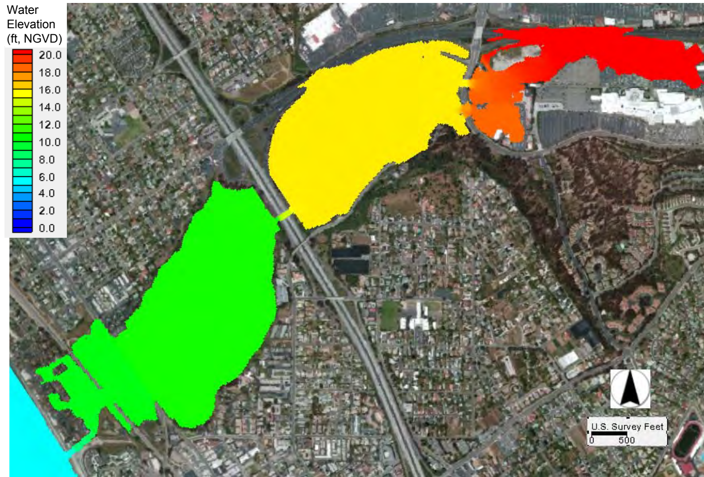
Figure 5.9 Maximum Water Elevations under Freshwater Alternative during a 100-Year Storm in Year 2050
