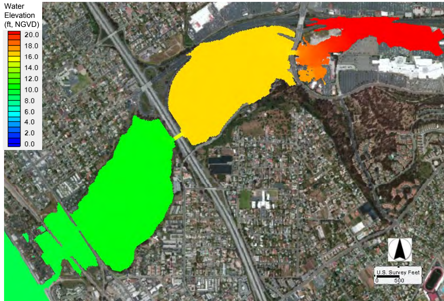
Figure 5.18 Maximum Water Elevations under Hybrid A during a 100-Year Storm in Year 2100
