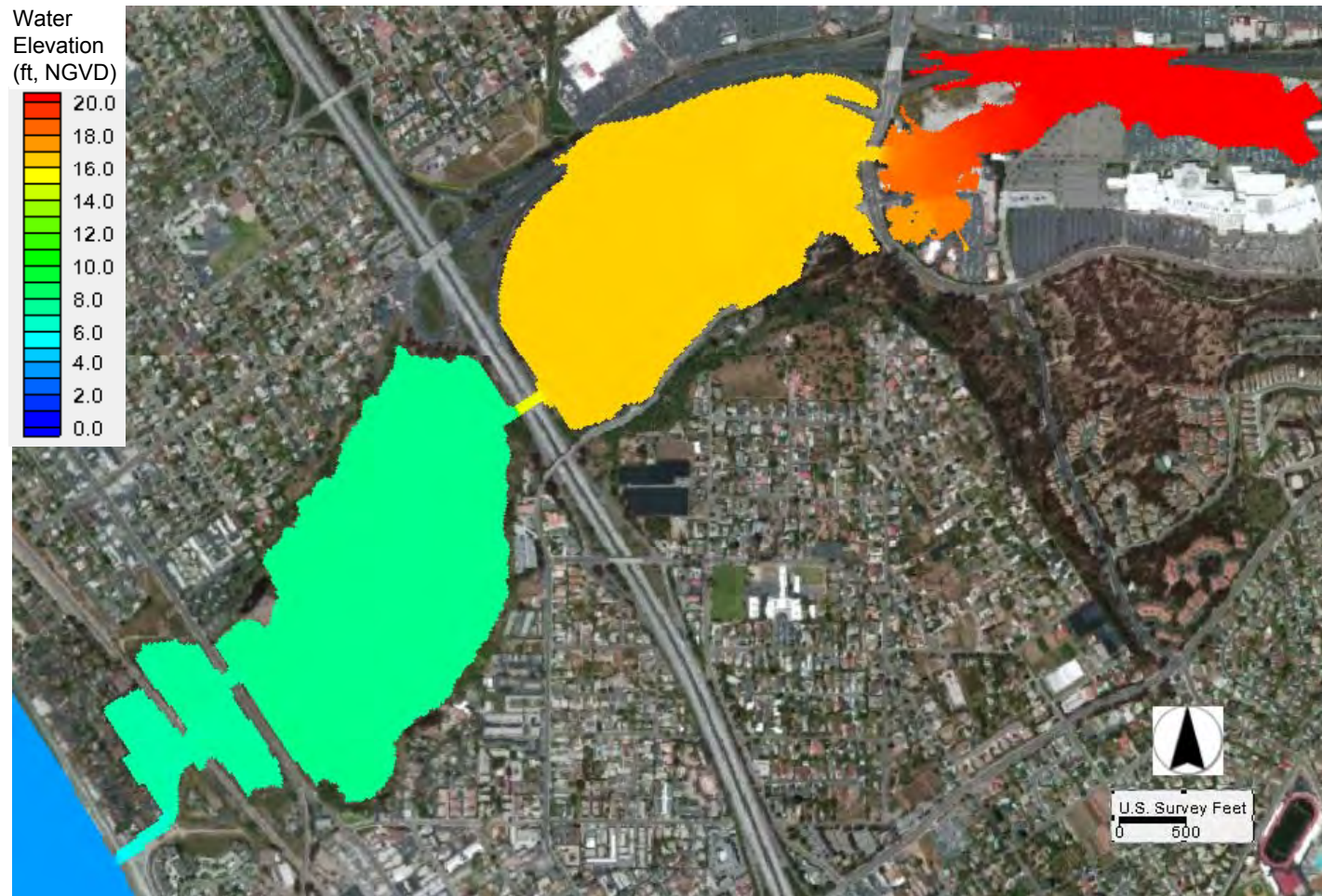
Figure 5.20 Maximum Water Elevations under Hybrid B during a 100-Year Storm in Year 2015
