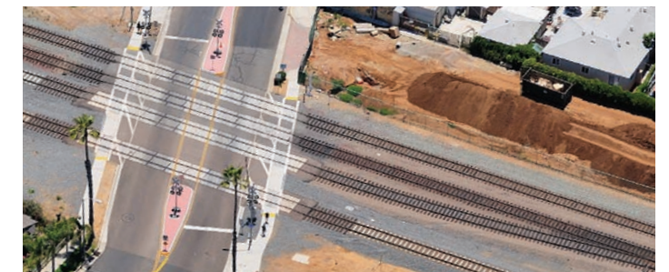
The medians at Wisconsin Avenue will be lengthened by the OTC Platform Improvement and Coastal Rail Trail projects, which will support a future Quiet Zone in the area.
