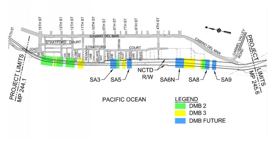
In DMB 2 & 3 we installed 200 piles in areas as shown above
