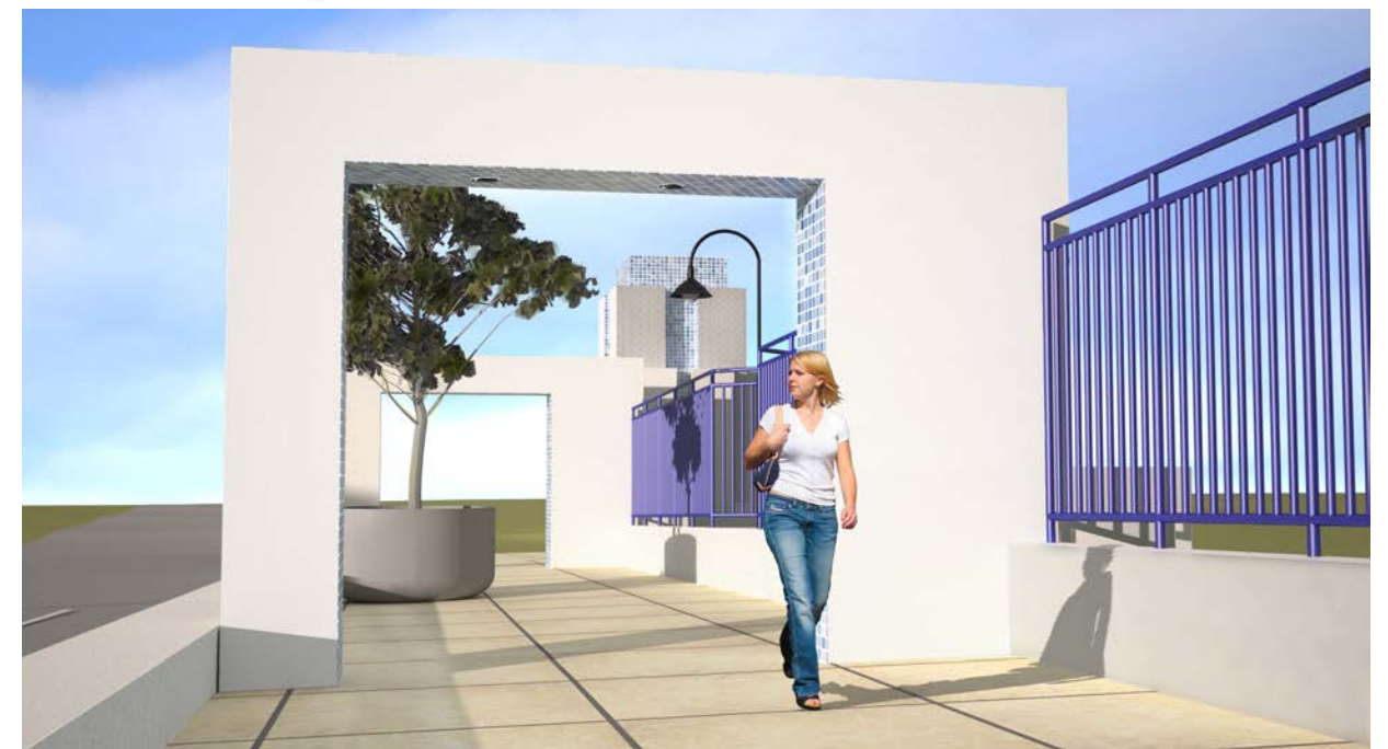
View of pedestrian crossing featuring the enhanced paving, tree planters and light fixtures enclosed between a decorative fence and low profile barrier adjacent to the roadside.
