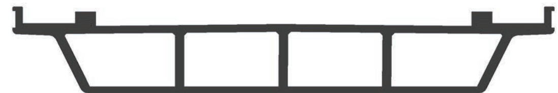
Coastal Mesa bridge deck section
