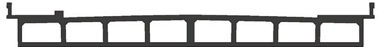
Northern Urban bridge deck section
