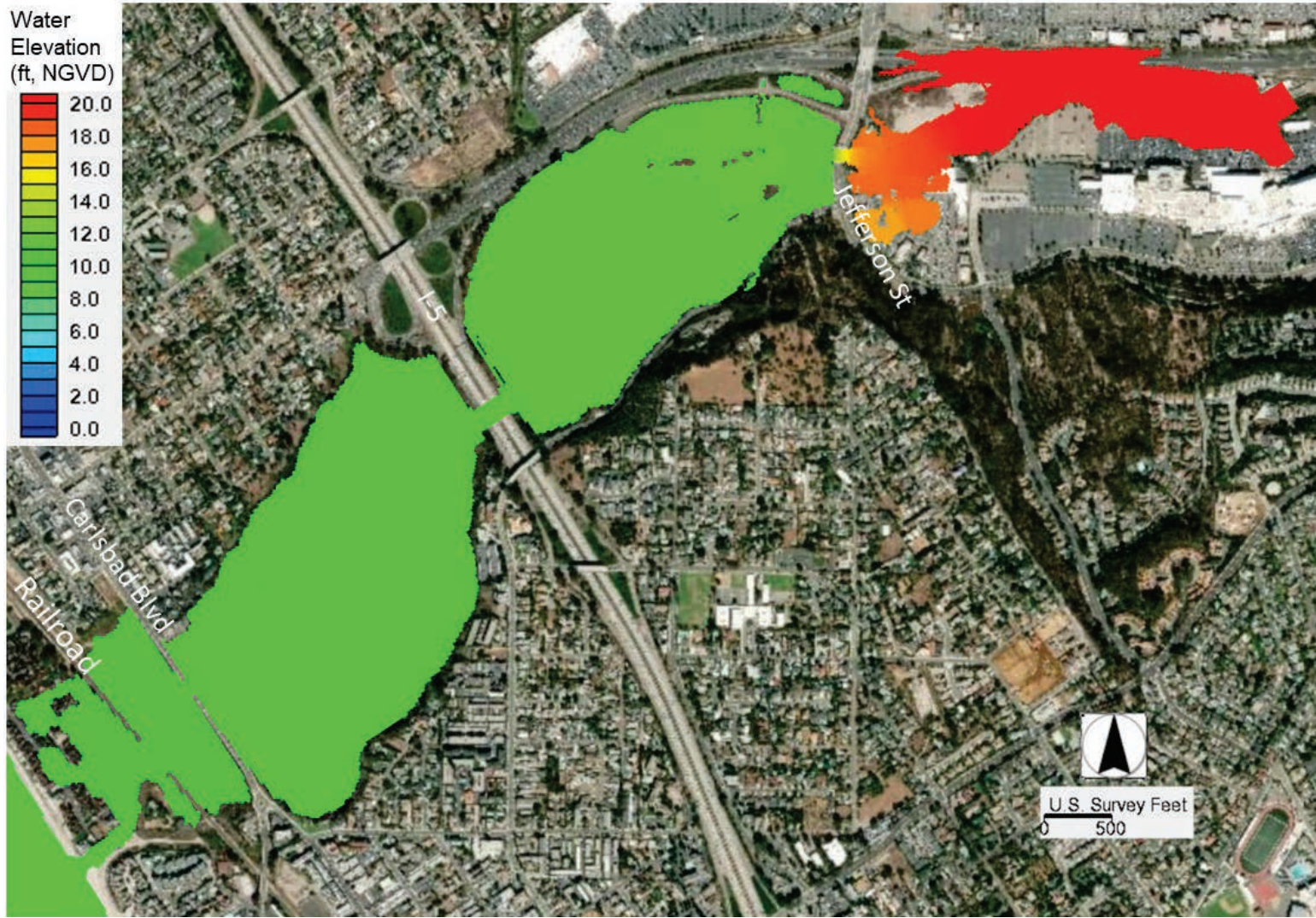
Figure 7 Maximum Water Elevations Under Modified Saltwater Alternative During a 100-Year Storm in Year 2100
