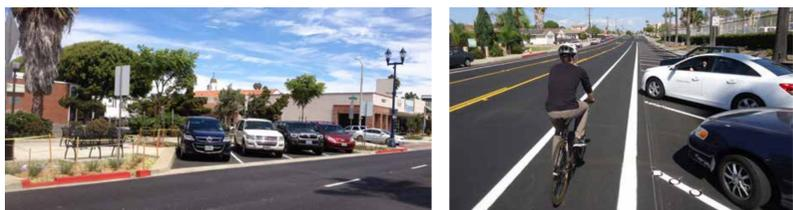
Back-in angle parking (also known as reverse angle parking) is a type of parking where cars back into their spots rather than pulling in, allowing them to make eye contact with oncoming traffic when exiting the parking space. Back-in angle parking improves the visibility of approaching traffic and people riding bikes, and increases the ease of loading cargo into the vehicle's trunk/bed.
