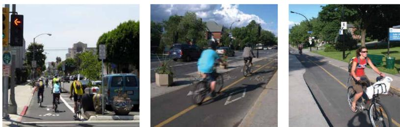
A separated bikeway is a one-way or two-way bike facility that is physically separated from vehicular traffic and distinct from the sidewalk. They can be separated by a curb, a median, parked cars, bollards, or other barriers. The physical separation creates a safer and more comfortable experience for people riding bikes that is attractive to a wider range of riders.
