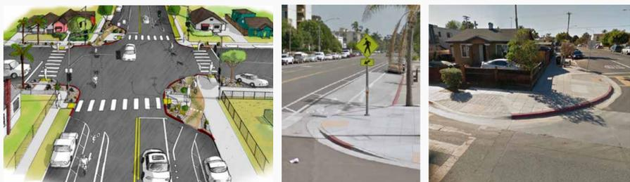
Curb extensions and bend-outs visually and physically narrow the roadway by extending the curb – pedestrian and bicycle queuing space – outward at intersections. By extending into intersections and providing refuge areas for people walking and biking, these features increase the visibility of people walking and biking, improve sight distance for people driving, encourage slower turning speeds, and shorten crossing distances.
