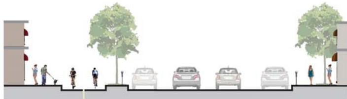
Potential 10' Cycle Track 5' Planted Side Median 8' Parking Lane 10' Travel Lane 10' Travel Lane 8' Parking Lane 52' Curb-to-Curb
