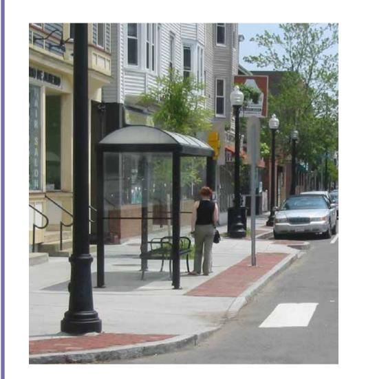
Bus bulb-outs are curb extensions that align the bus stop with the parking lane. Like curb extensions, bus bulb-outs can help shorten pedestrian crossing distances, while also helping buses move faster and more reliably. Examples of where bus bulb-outs would be located are the intersections of University Avenue with Vermont and Richmond streets.
