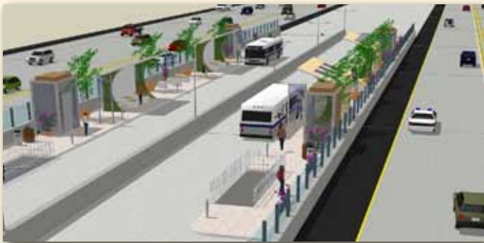
In-line transit stations will be constructed in the center of the freeway, providing convenient access to the Express Lanes and reducing congestion by eliminating the need for buses to exit the highway.
