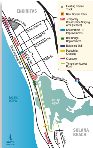
The project will add 1.5 miles of second main track and replace an aging timber rail bridge on the LOSSAN coastal rail corridor between the cities of Encinitas and Solana Beach.
